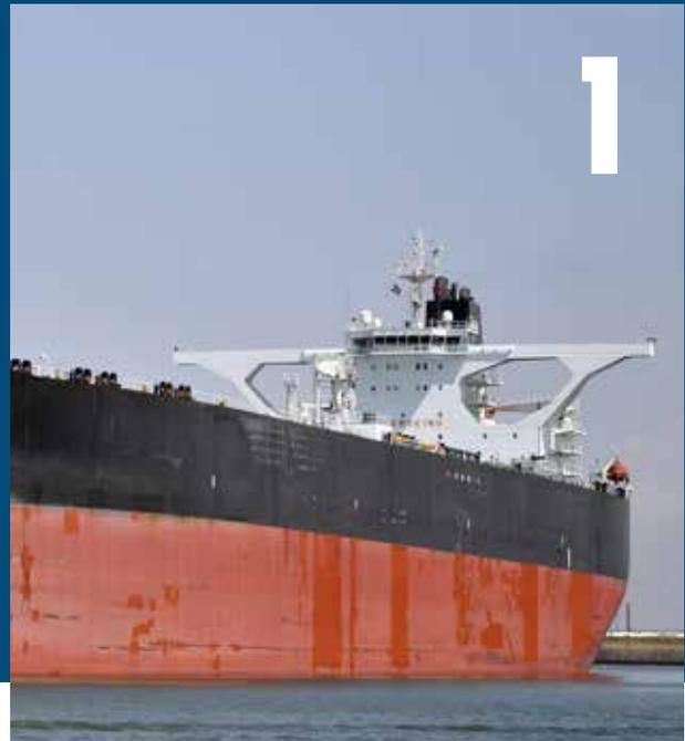
In general, to date the treatment or disinfection of ballast water is directly connected and in parallel with cargo activities in Port. This timing seems logical as cargo is discharged or loaded and the weight differential must be compensated by port water pumped to the ballast tanks. In reality this practice poses some operational challenges for high ballast dependent ships.
